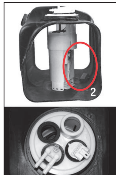
Improperly positioned fuel pump module assembly
